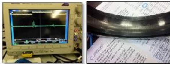
High Frequency Noise Fluting from Generated by VFD Common Mode Currents
